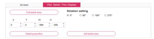
Set any part of the work area of the device to be mapped as the display area of the screen. The driver provides four modes for selection:
